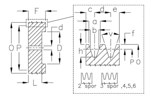
$\begin{array}{lll} D & = 83 \\ d & = 20 \\ F & = 120.0 \\ L & = 60 \\ Number of ribs = 6 \\ O & = 132.0 \\ P & = 125 \\ Type & = B \end{array}$
